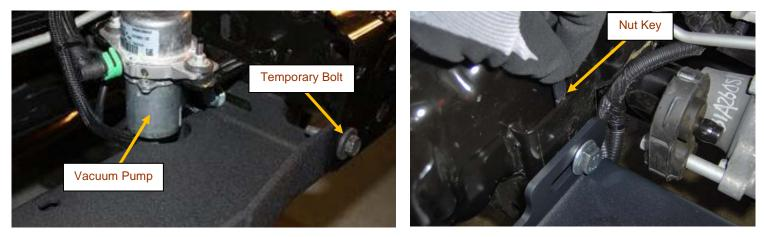
Align the front holes and clamp as shown in the image below. You can also use a bolt and a nut to temporarily clamp. Tighten and torque the back bolts using the 19 MM drive socket and ratchet as shown below – <u>Torque to 66.5 Ft.Lbs on each bolt.</u>
