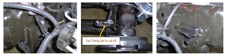
Using a 10 MM socket/wrench, assemble the vacuum pump relocation bracket to the winch plate using the 2 M6 bolts and washers provided.
