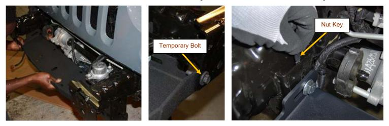
Align the front holes and clamp as shown in the image below. You can also use a bolt and a nut to temporarily clamp. Tighten and torque the back bolts using the 19 MM drive socket and ratchet as shown below - <u>Torque to 66.5 Ft.Lbs on each bolt</u>.
