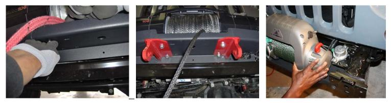
Check winch position alignment and clearance from the vacuum pump. Note the slotted holes on the plate to allow for side adjustment. If not a WARN Zeon winch, tighten and torque all the 4 bolts using a drive socket and ratchet - <u>Torque to 30 – 35 (Ft.Lbs) on each bolt</u>.
