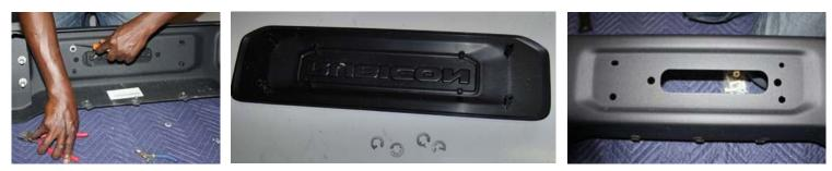
First widen the fairlead opening on the bumper following the steps below (making the slot "symmetric"): This step is a must for a centered winch setup ONLY. If you are doing an offset setup then skip this step and **go to step (B)** below.
