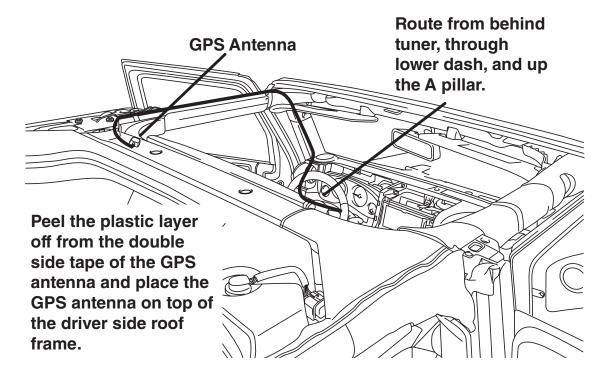
There is no way to integrate the factory SiriusXM tuner. Once the radio is removed, the factory SiriusXM is removed. As the title states, SiriusXM requires a tuner sold separately. This diagram shows how to integrate the antenna connection.
