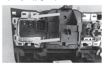
16 Connect the camera interface module to the violet factory camera plug and put it in right side of radio cavity. Dip switch 1 will need to be moved down for the Gladiator JT.
