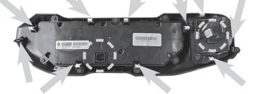
2 Unsnap the 6 clips and remove the knee panel under the steering wheel using a panel removal tool.
