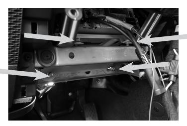
12 Attach the factory Power module to the bracket using the OEM screws. This is what the power module will look like for the Gladiator JT.
