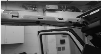
14 For vehicles with heated seats or the power inverter the bracket for the module needs to be removed. Remove the (4) 10mm screws to remove the bracket. Then remove the (2) 8mm screws lower and the (2) 10mm screws top to remove the module.
