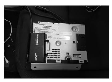
9 Use the factory speed clips from the bracket that was removed from the vehicle and attach them to the Power Inverter bracket. For the Wrangler JL use the 2 holes circled in black. For the Gladiator JT use the 3 holes pointed out by the arrows.
