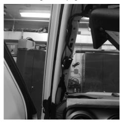
3 Mount GPS antenna near driver side B-pillar as illustrated on page 18 and run the cable to the knee panel.
