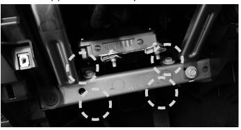
16 Remove the A pillar by removing the (2) 8mm screws and unclipping the panel. The screws can be exposed using a panel removal tool.
