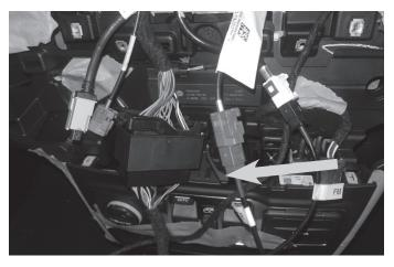
17 Attach the Maestro to the main harness and tuck it in left side of radio cavity.
