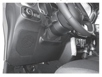
4 Unsnap 10 clips, unplug the 2 harnesses, and remove HVAC panel using a panel removal tool.
