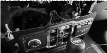
17 Loosen the clips around the top panel visor area.
