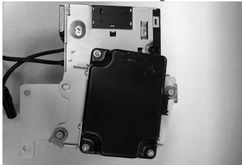
13 Use (4) OEM bolts to secure the X409 source unit tuner bracket to the vehicle. If the vehicle is equipped with the power inverter it will mount behind the 2nd cross bar.
