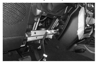
6 Attach tuner bracket to tuner using (4) M5X8LMM supplied screws.
