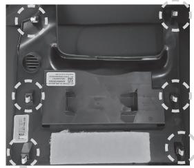
5 Locations of the clips and harnesses of the HVAC controls from the previous step.
