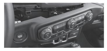
6 Use #2 Phillips Screwdriver to extract (2) screws from the bottom of the radio bezel.
