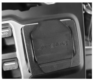
22 Attach the display unit to the display bracket using the (4) M5X8LMM supplied screws.
