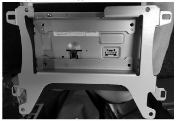
24 Plug in the bezel and and reinstall all the factory panels.
