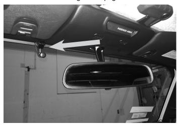
4 Route radio cables including Radio Main, Sirius XM, FM, and Aux in main harness and also the display cable from radio cavity to knee panel.
