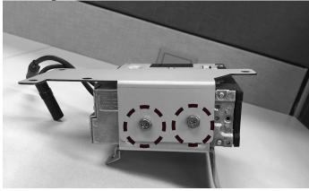
10 After attaching the factory speed clips this is what the bracket will look like for the Wrangler JL.
