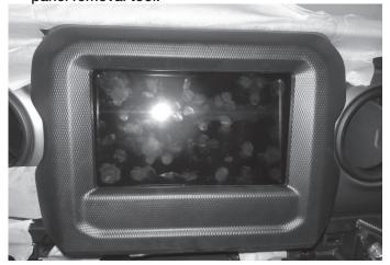
9 Use #2 Phillips Screwdriver to extract (4) screws from head unit. Disconnect and remove the radio.
