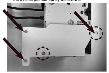
8 For vehicles with heated seats or the power inverter attach the Power Inverter bracket using the supplied (2) M5X10LMM screws and lock washers. This will mean you will not use two of the M5X8LMM screws from the previous page. These two screws are slightly longer and can make it through both brackets.
