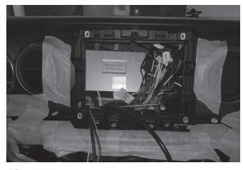
18 Run chime speaker harness from Maestro module to behind the glove box and attach there.
