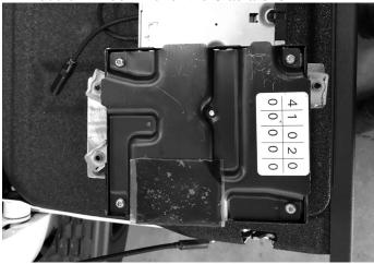
14 At the knee panel, connect the main harness, display harness, GPS antenna, microphone, USB cable, HDMI, FM adapter, and other adapters to X409 source unit and secure them.
