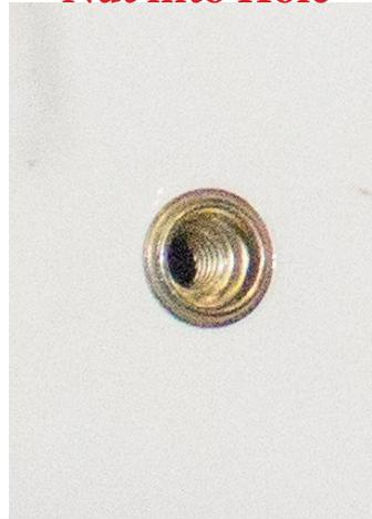
**Tighten Rivet Nut as Shown**
