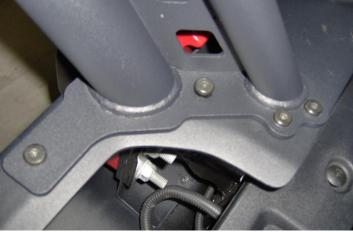
Alignments and make sure the bar/hoop is seated flat on the mounting surface. Now tighten the lower M8 hex bolts of the reinforcement brackets, 1 on each side.
