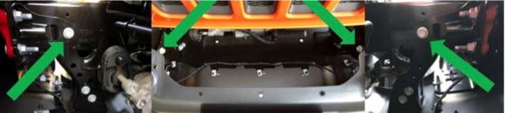
\*\* The reinforcement bracket's top bend goes to the inside. \*\*
