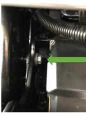
Picture of bolt to be removed with winch plate installed.
