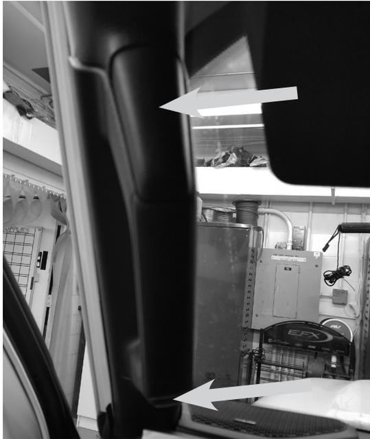
**13** Loosen the clips around the top panel visor area.
