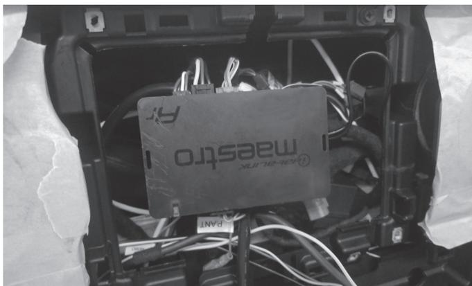
**8** Run chime speaker harness from Maestro module to behind the glove box and attach there.
