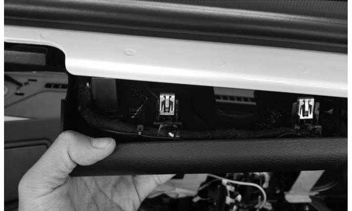
**14** Unclip 7 clips and remove the center media stack.
