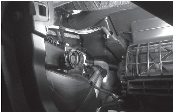
**6** Connect the camera interface module to the violet or red factory camera plug and put it in right side of radio cavity. Dip switch 1 will need to be moved down for the Gladiator JT.
