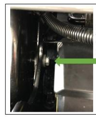
Picture of bolt to be removed with winch plate installed.
