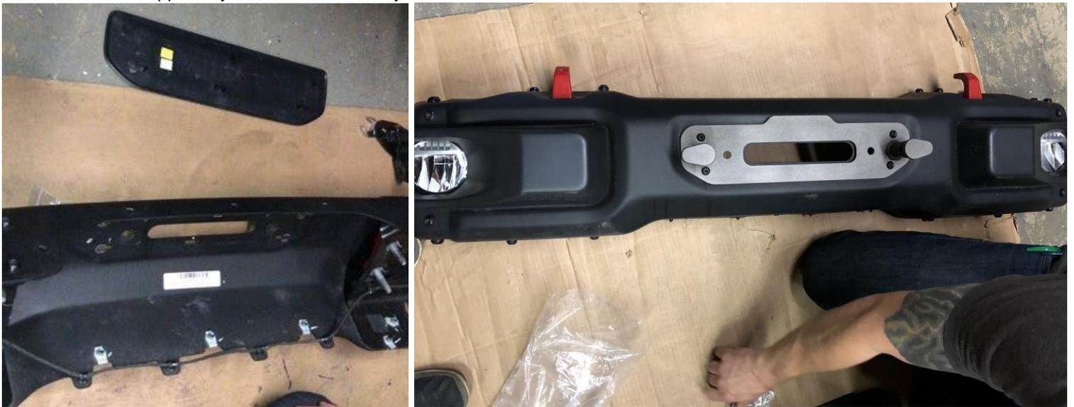
**(18) INSERT SPACER PLATES TO BUMPER STUD BOLTS:**
