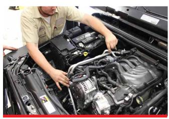
Remove aluminum coolant pipe assembly from passenger side of engine.
