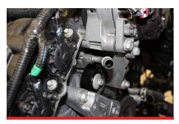
**F.** Using the box end of a wrench, gently rotate the coolant fitting upwards towards alternator as shown.
