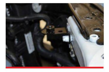
**C.** Attached modified bracket to mounting stud in front of original location as shown.
