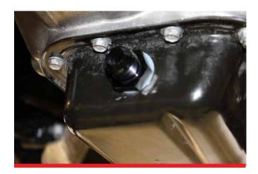
K. Attach oil drain hose to oil pan. Make sure you hold base of fitting so it does not rotate while tightening.
