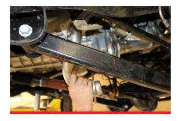
C. Attach passenger pipe to engine and turbo feed pipe.
