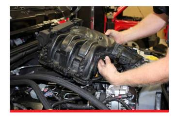
**A.** Attach all o-rings on the lower intake manifold.
