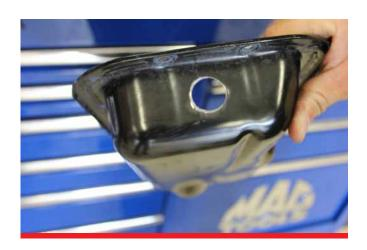
E. Using a hole saw, drill a 7/8" hole as shown. Clean any burrs so surface is flat.
