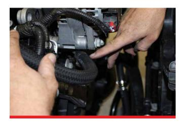
C. Install supplied heater hose to fitting near alternator and attach to driver side heater core tube.
