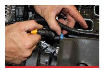
**G.** Remove safety tab on fuel supply connection.
