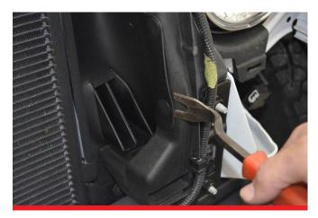
**C.** Remove air diverters and discard. We found this type of tool works well.
