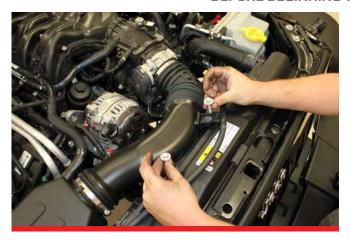
**A.** Remove entire factory air intake system including lower box portion under air filter.
