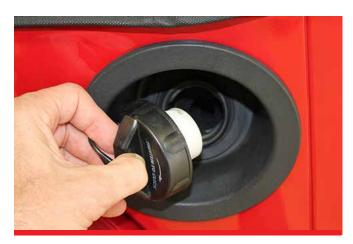
**F.** Loosen vehicle fuel cap to relieve pressure in fuel tank.
