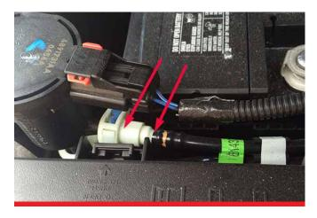
F. Install supplied vacuum hose assembly to blowoff valve, intake manifold, wastegate and purge control valve per diagram. (Route away from any direct contact with heat source) Use zip ties where necessary. (add pic of diagram here)
