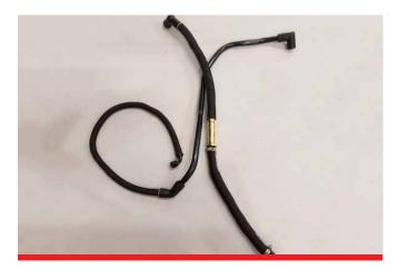
F. Attach to the supplied air filter hose as shown. This will connect to the fitting on the air filter.
