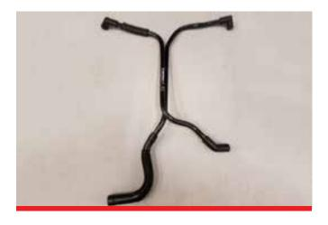
**A.** A. Remove the factory PCV lines shown . This shows their orientation in the vehicle.
