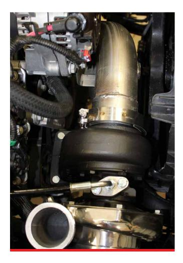
**G.** Tighten turbocharger to flange. Make sure air filter does not contact surrounding plastic when tight.
