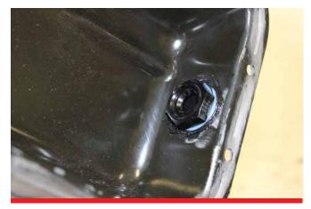
**G.** Attach oil drain fitting as shown with washers and sealant on both sides between washers and oil pan.
