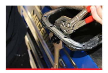
**H.** Secure fitting to oil pan. Clean residue with dry rag.
