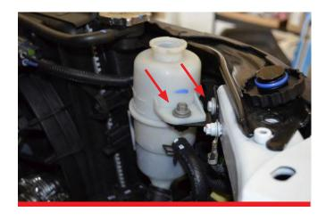
**A.** Remove the bracket that holds the power steering reservoir to the radiator core support.
