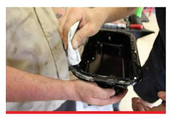
J. Apply sealant to oil pan surface going around inside of bolt holes.
