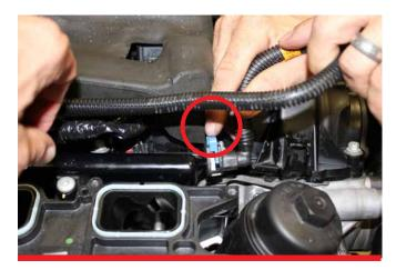
**C.** Reinstall fuel feed line and safety lock.
