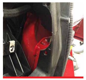
**D.** Clearance core support on both passenger and driver side for silicone hoses as shown.
