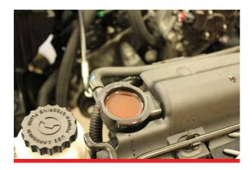
**C.** Top off cooling system and put radiator cap back on.
