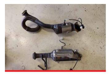
E. Remove left and right cat equipped pipes.
