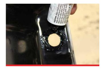
**F.** Apply sealant between the nylon washer and the pan surfaces.(both sides)
