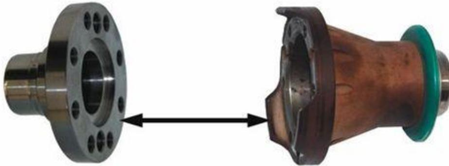
**Measure from lip of flange on transfer-case out-put to face of flange at differential.**
