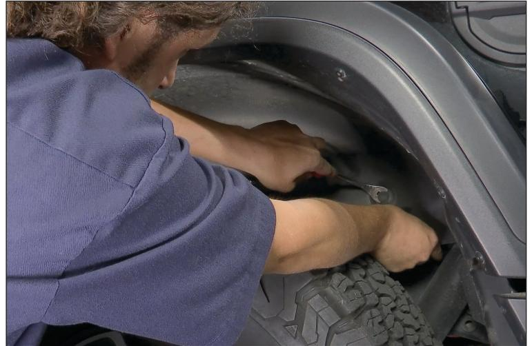
2. With the inner liner loose now you can remove the entire fender. Grab the fender and pull the fender away from the body. It's attached with clips. When pulling it away the clips will probably break but its okay your not reusing them. Start pulling from one corner and work your way to the other side of the fender.
