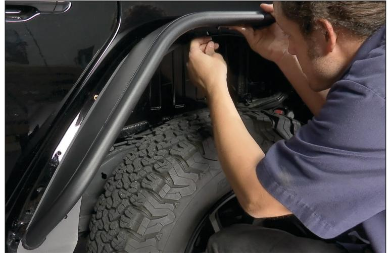
11. Now fully tighten hardware in a alternating pattern. Avoid using power or air tools. The last button head towards the rear of the fender is tight to the tube, it requires a short Allen head key to hold and tighten. This completes the install.
