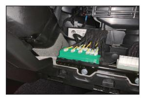
11. Take the supplied bypass cable shown and connect the white connector as shown at the red arrow location. Route the cable along the base of the dash towards the OBD connector. Use zip ties to secure it out of the way.
