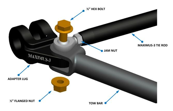
Do the same for the other side. Make sure the Tie Rod ends are adjusted the same length/threads as a start.
