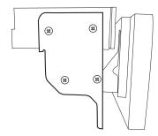
6 Route the key harness through the top-left side of the i509 source unit. Mount the i509 source unit using (4) 7mm factory screws.
