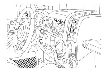
6 Extract (2) 7 mm screws from the factory radio bracket and remove it.
