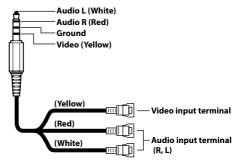
Configuration commercially available 4-pole mini AV plugs is not standardized.
