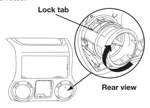
4 Mount the microphone as illustrated and run the cable to the radio cavity.
