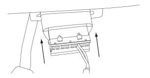
2 Remove the vents from the radio section on the OEM dash panel by pressing down on the lock tab and turning right. Mount vents on to the i509-WRA-JK bezel.
