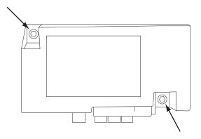
3 Secure the Uconnect® module to the original location using the 7mm bolts.
