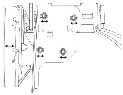
Adjust the side brackets as needed when either side is protruding or not flushed.
