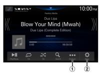
① Displays up to 15 labels obtained from iDataLink. A generic list, popup window, or current source screen is displayed by touching the Custom1 to 15 buttons. The screen that is displayed is determined by iDataLink.
