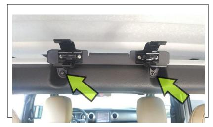
Remove three factory torx bolts using a T-25 torx bit. Two are in the rear cargo area. The third bolt location is above the rear seats (other side of the sports bar)
