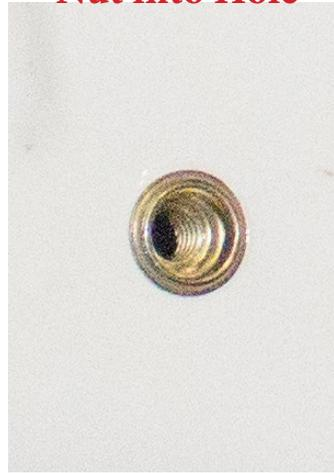
**Tighten Rivet Nut as Shown**
