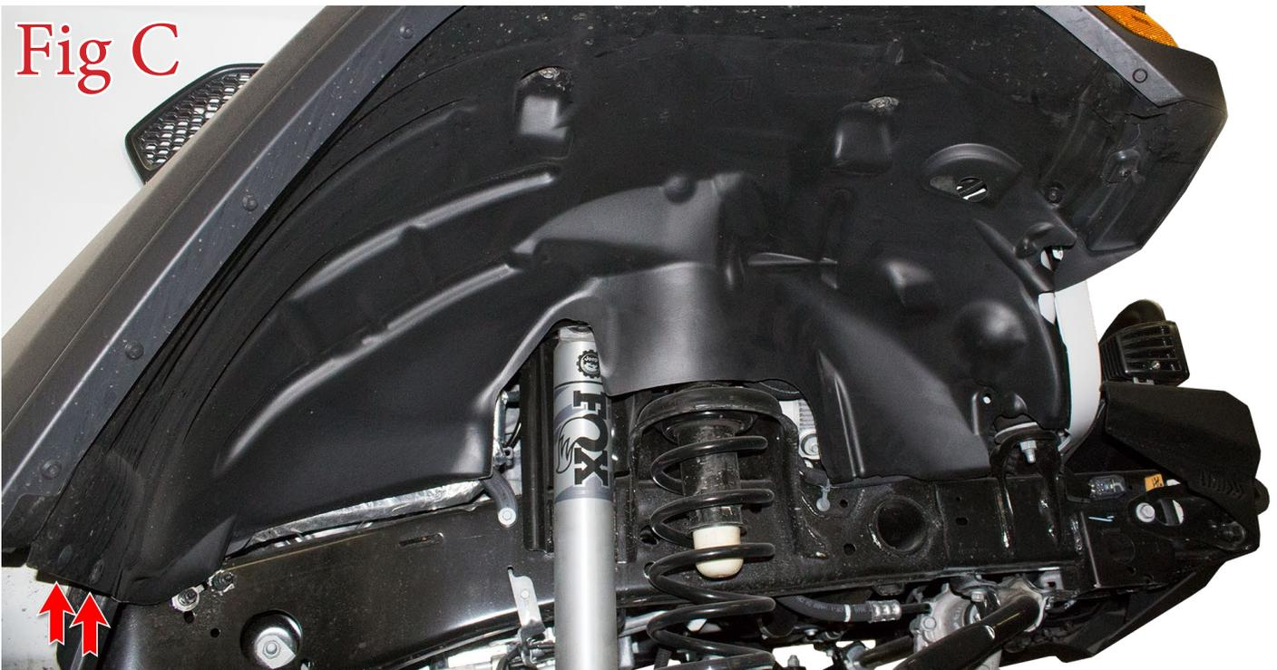
4. Release the series of push rivets that hold the inner liner to the fender on the outer edge of the wheel well. (Fig D)
