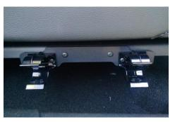
If your JK does not have matching holes on the seat rail as with older JK's, align the bracket to the existing hole, mark and drill a second hole to mount.
