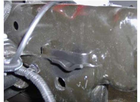
Using a 10 MM socket/wrench, assemble the vacuum pump relocation bracket to the winch plate using the 2 M6 bolts and washers provided.
