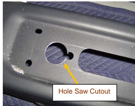
Carefully cut on the lines you marked using a cut off wheel or a grinder as shown below. De-burr the edges using a file. Paint the edges for rust protection using a small brush or spray can.
