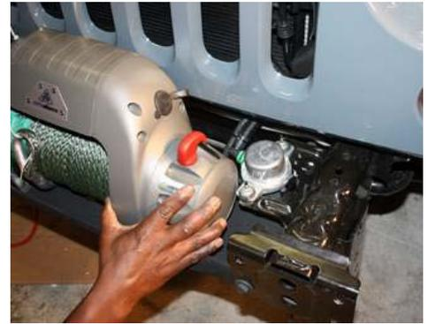
Check winch position alignment and clearance from the vacuum pump. Note the slotted holes on the plate to allow for side adjustment. If not a WARN Zeon winch, tighten and torque all the 4 bolts using a drive socket and ratchet - Torque to 30 – 35 (Ft.Lbs) on each bolt.
