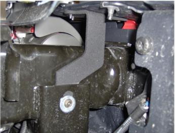
Install the light brackets using the factory M6 bolts you removed in Step 2 and the 4 M6 nuts provided, 2 on each bracket (you do not need the nuts for non-winch install).
