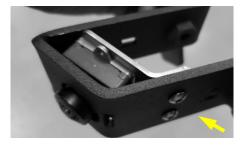
Feed the camera wire through the back of tire mount to the front.
